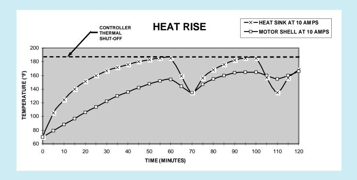
The RV Aquajet II Pump is capable of sustaining continuous running for approximately 1 hour, as shown in the above Heat Rise graph. The Speed Controller is equipped with an auto reset thermal protector that will shut down the system, allowing the components to cool. After approximately 10 minutes the pump will restart.
